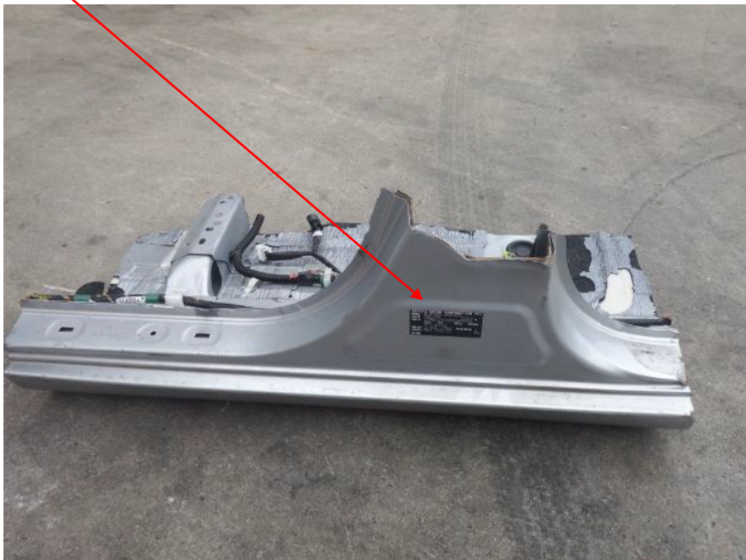
14.4 Figure 11: Section of sill and 'B' pillar from a stolen Toyota RAV4, build plate attached
