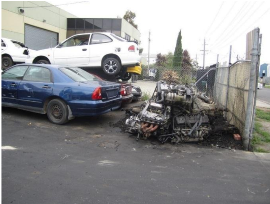
22.2 Figure 26: Completely non-compliant worksite, vehicle bodies stacked unsafely
